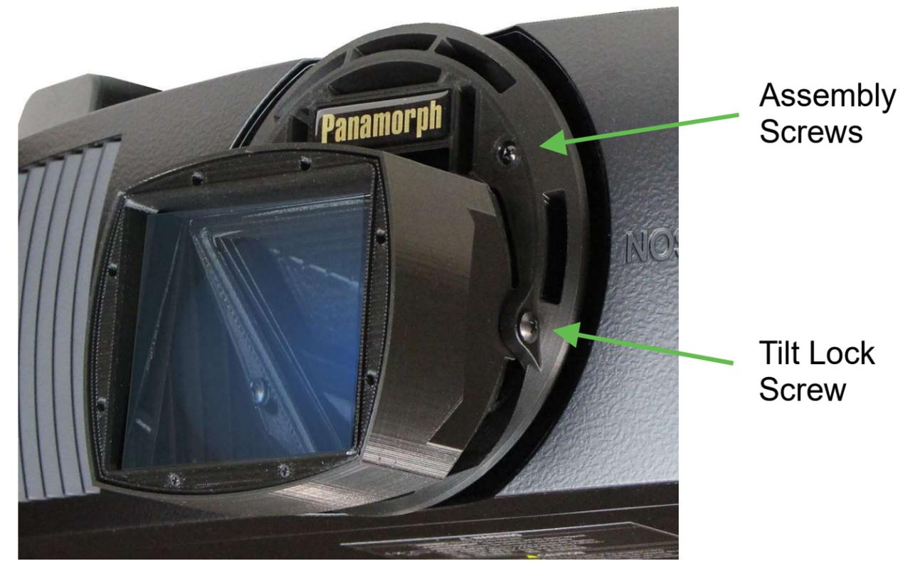
**2 PREPARE THE PROJECTOR.** Make sure the projector lens is horizontally centered in its opening (ie little or no horizontal lens shift). Adjust the projector roll, tilt and/or yaw so the projector test pattern lines are square to the screen edges and the test pattern is centered on the screen. Then **show a 2.4:1 movie**. Use the Epson “Aspect” button on the remote to select “Anamorphic Wide” and make sure the projector lens is clean and as dust free as possible.
