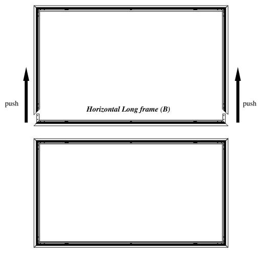
8. Make sure all four corners are properly in place to form a perfect square. Then fasten the four angles with the *M5x15 Screws* (*H*).
