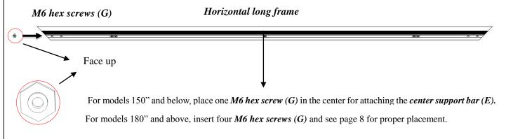
5. Insert the *elbow joint* (A) into each end of the *horizontal frames* (B) as shown below.
