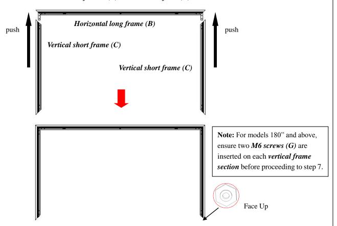
7. Join the remaining *horizontal long frame* (B) with the frame built in the previous steps as shown below.
